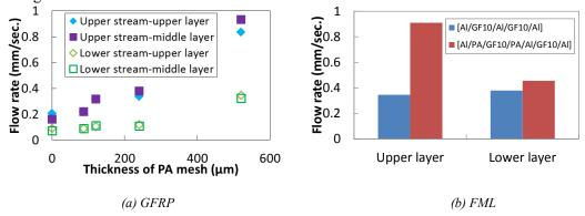
Figure 2: Results of flow rate of resin during VaRTM process.
