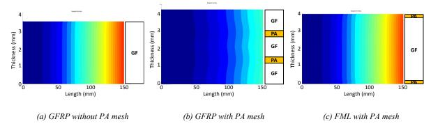
Figure 3: Simulation results of the shape of the flow front.
