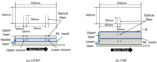
Figure 1: Set-up of fiber optic sensors.
